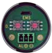
Thermalert 4.0 supports 2-wire loop
